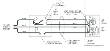
DUAL SWITCH ELECTRICAL WIRING TO FIREPLACE RECEPTACLE
